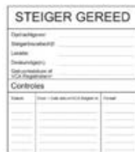
Completed scaffold tag in the tag holder, as soon as scaffold is completed
